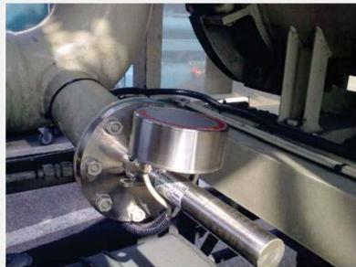
Take the guesswork out of product switching. A faster and more accurate inline density meter tightens control of pushed products and delivers true density and API. Simple to automate, it ensures the correct product is transferred and reduces slop tank volume, blending and residence time.
