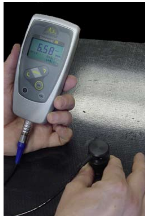
Measurement of Composite Thickness with Steel backing plate.
