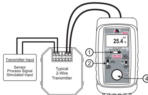
The Meriam Model M334 supplies a nominal 24 volts DC at 24 mA to the 2 Wire Transmitter. The current passed by the transmitter will be accurately displayed by the Meriam Model M334. Calibrate the transmitter in the usual manner and disconnect the Meriam Model M334.
